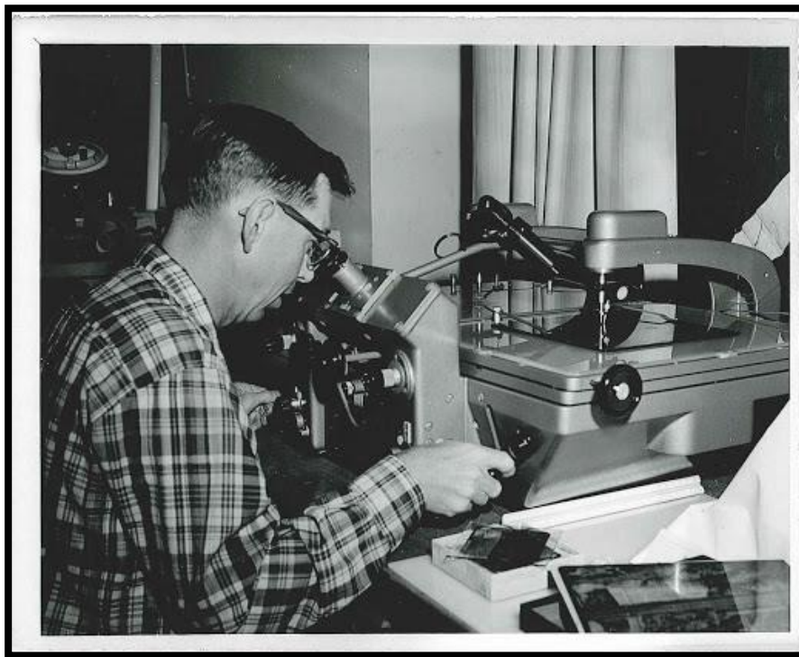
Figure 2 : Analog renderer photogrammetry [10]
