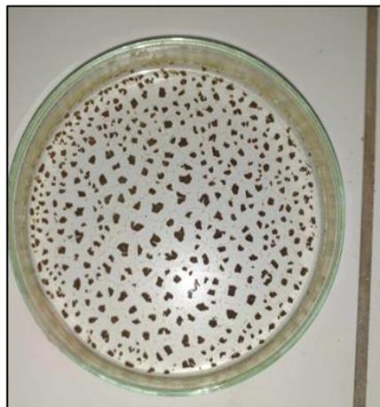
**Figure 18:** Nanoparticules de ZnO.
