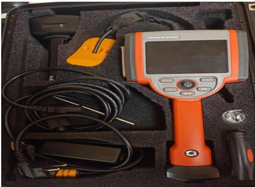
**Figure IV.14: Photo Boroscope Olympus [72] .**
