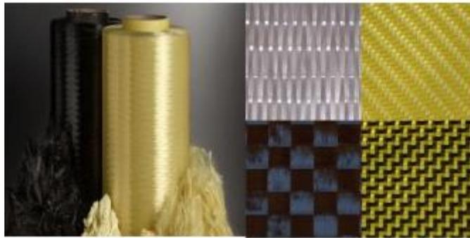
Figure II.5: Fibre aramide. [16]
