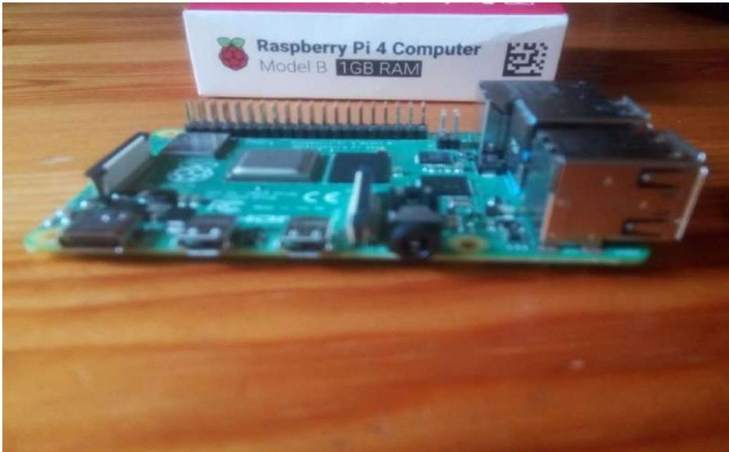
**Figure3.7** : la raspberry pi 4 model B 1GB RAM
