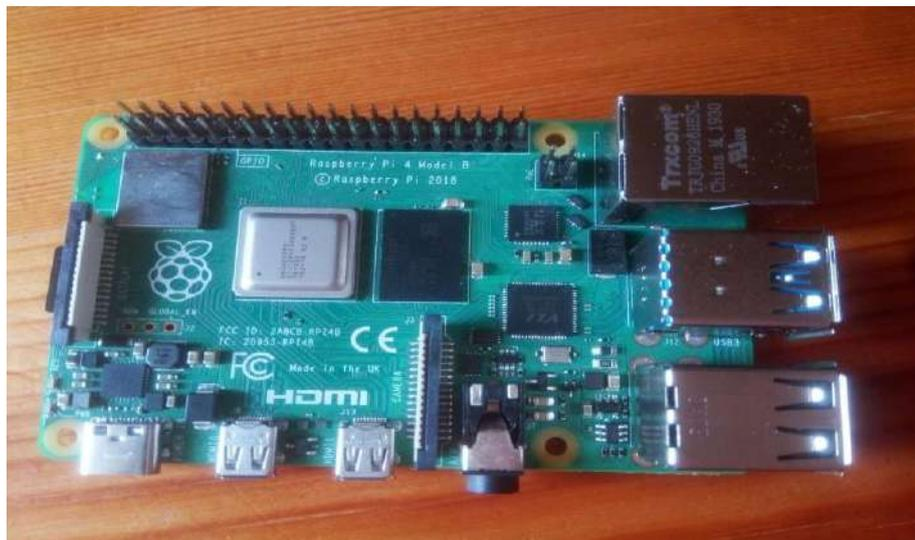
Figure3.3 : la raspberry pi4 model B
