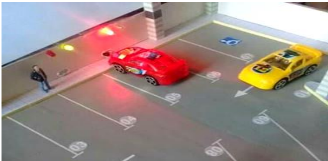
Figure III. 12: Place occupée (LED rouge) et place libre (LED vert)
