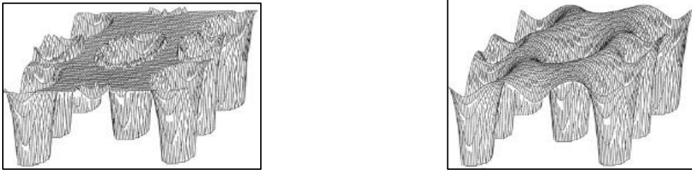
Figure III. 3 (a) Potentiel muffin-tin, (b) Potentiel complet.
