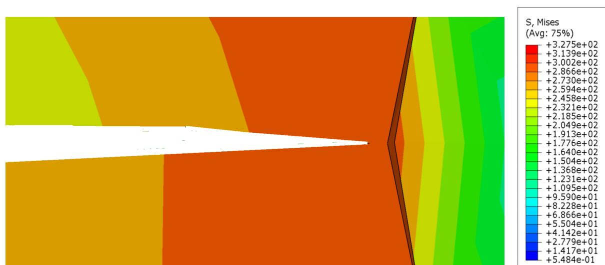
Fig. IV.5 Interaction fissure-inclusion ( $a=10\mu\text{m}$ ,  $d=0.1\mu\text{m}$ ,  $\Delta T=300^\circ\text{C}$ )
