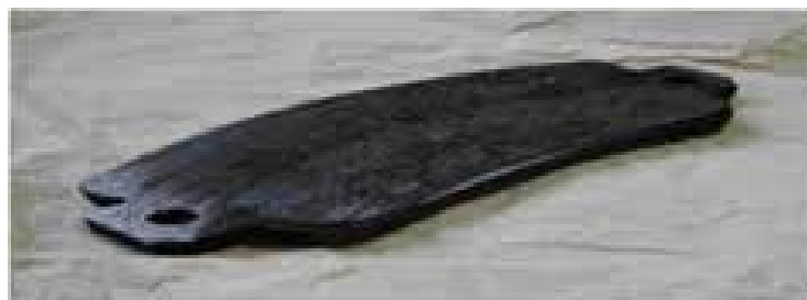
Figure IV-17 : Usure excessive des plaquettes
