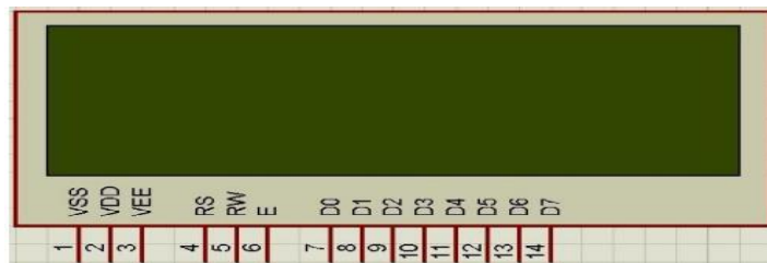
Figure III.3: afficheurlcd lm016 16x4
