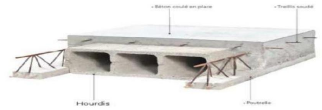
Figure I.10 : plancher a corps creux
