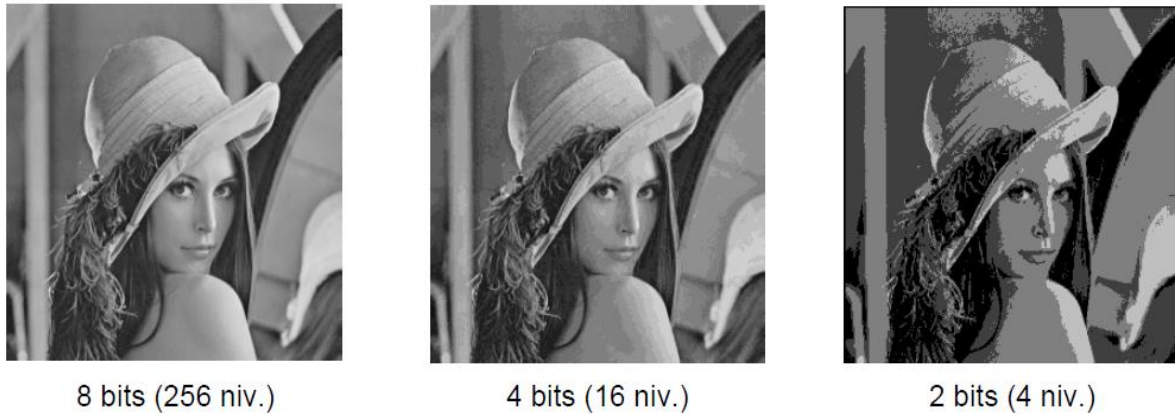
Figure I 2 Exemple de quantification sur 8 bits, 4 bits, 2 bits
