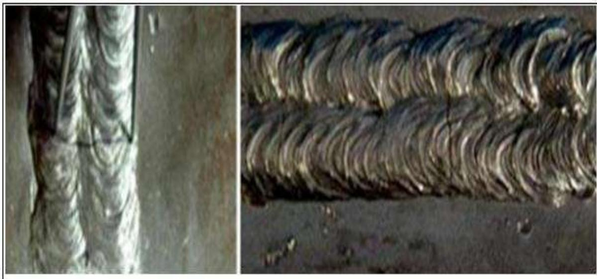
*Figure 26: fissure transversale[21].*
