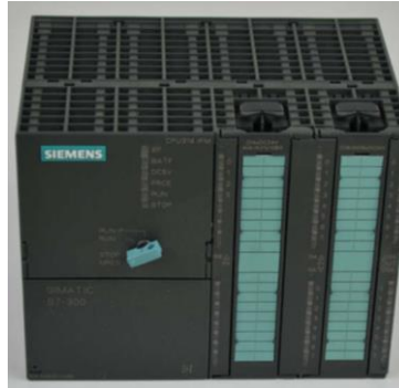
Figure III-3 : La CPU 314[W16]
