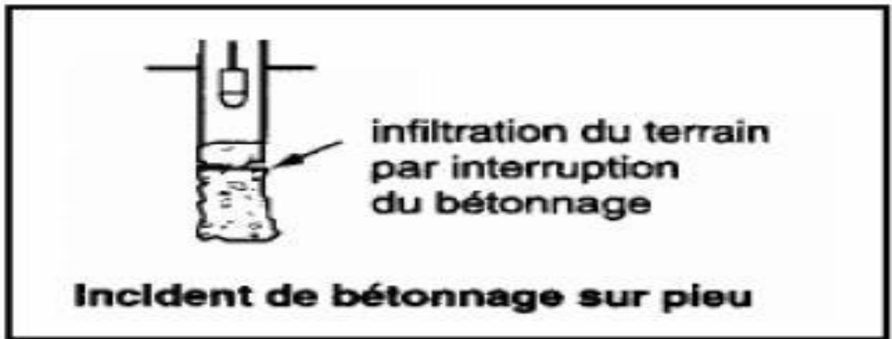
Fig.1.12 incident de bétonnage [2]
