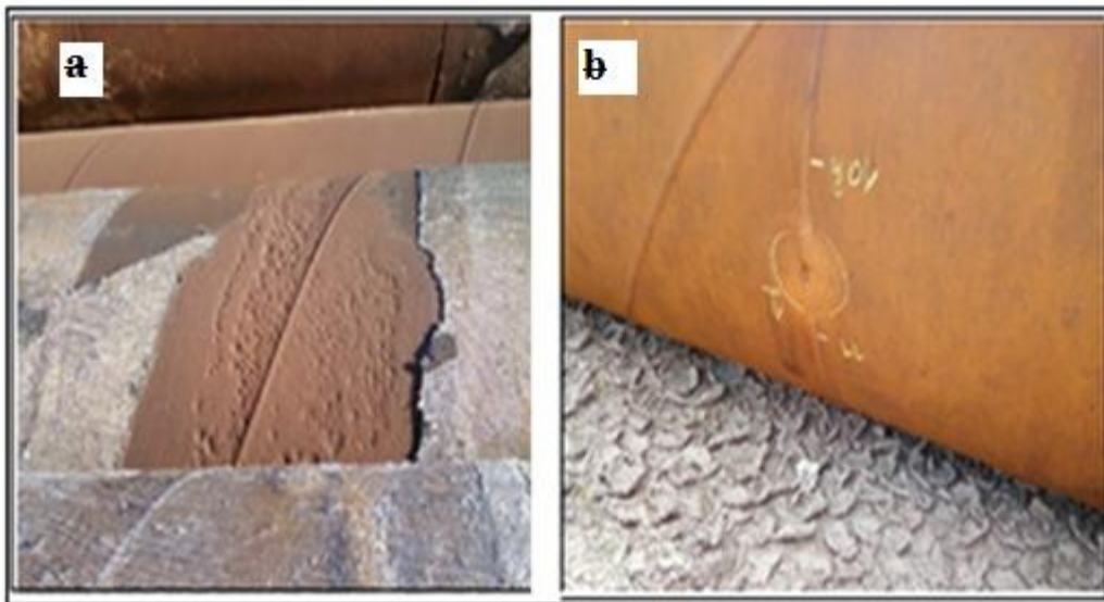
Figure 16: Types de corrosion[17]
