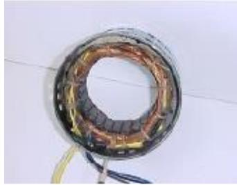
FigI-2 Stator de la machine asynchrone
