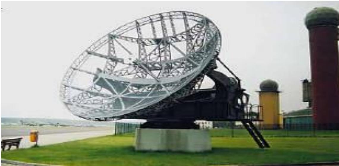
**Figure II.3:** Giant Würzburg radar [4]
