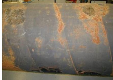
*Figure II-13 : Corrosion due aux infiltrations et parties saillantes (cordons de soudure)[10]*
