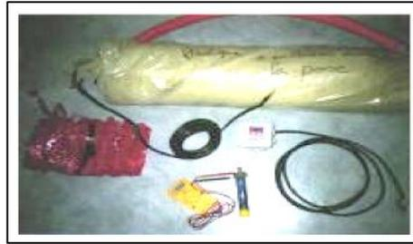
Figure II-24: ANODE SACRIFICIELLE [29]
