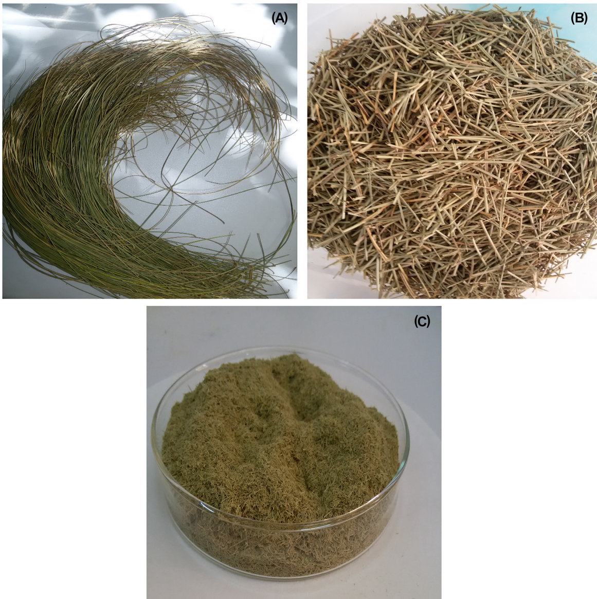
Figure 1: Physical preparation of the alfa fibres: (A) the alfa stems gathered; (B) the cut alfa stems; and (C) the alfa fibres collected from a 250 \mu\text{m} diameter sieve.
